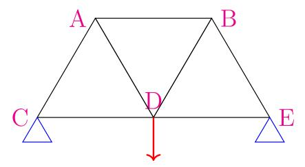
Figure 75 A simple truss
