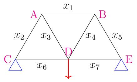
Figure 76 Variables for the truss
