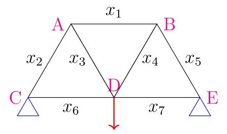
Figure 78 Variables for the truss
