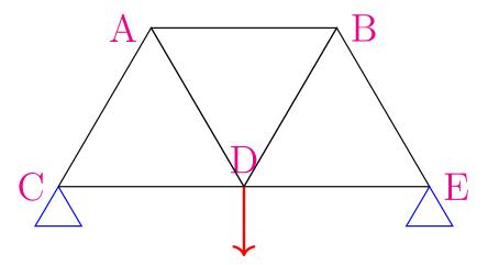
Figure 70 A simple truss
