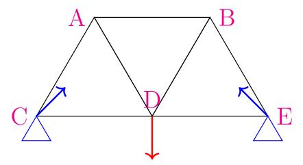
Figure 77 Truss with normal forces
